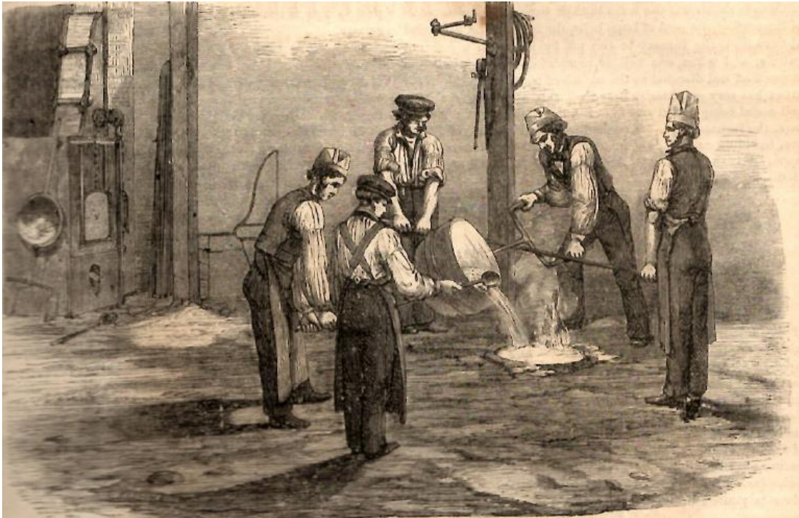
Figure 7: Pouring the Metal in the Mould: Illustrated Magazine of Art (Volume II 1854) page 293: as illustrated by I E Waldeck (15.0cm by 9.8cm)
