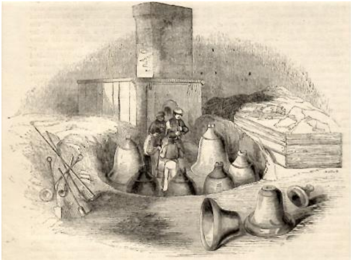
Casting Pit of a Bell-Foundry: Illustration from Knight's Pictorial Gallery of Arts , circ 1860 (13.0cm by 10.0cm)
