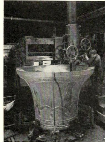
When the metal is cold the mould is removed and the newly-cast bell is taken from the core. The bell is then given its correct tone by the machine seen in this picture.
