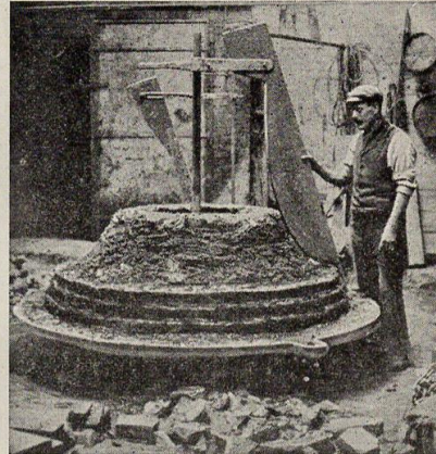
2. The core shaped like the inside of a bell is made from "foundry mud," and here we see the work started,
