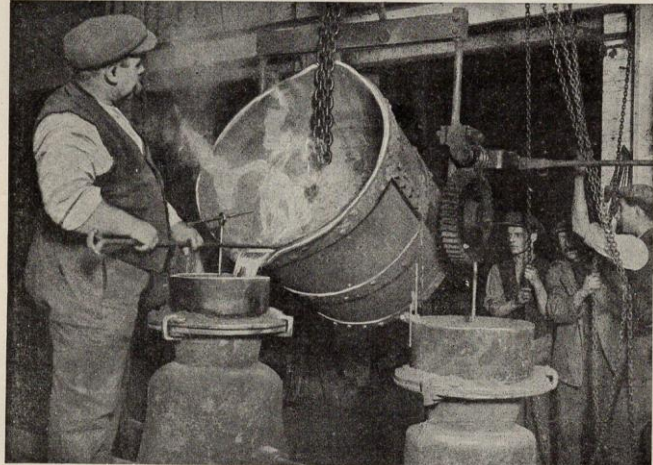
10. The cauldron containing the molten metal is swung by a crane to the spot where the mould and core are standing ready to receive the metal; and the cauldron, being turned by machinery, pours the metal into the top of the mould.
