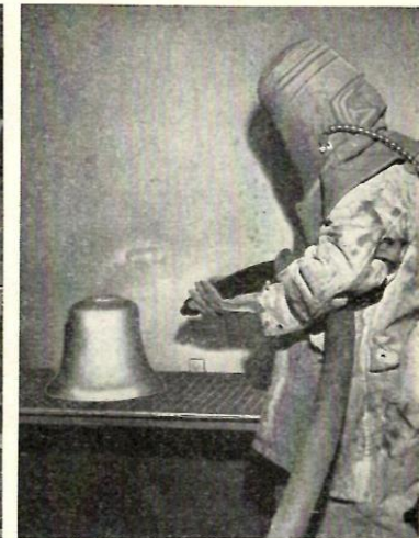
The final process is the smoothening of the surface by sandblasting, and the worker who does this has to be encased in a special dress to protect him from the dust.
