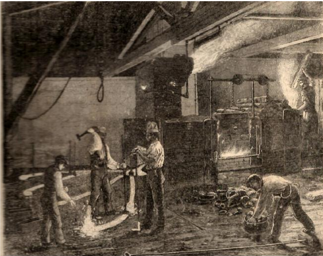
Figure 8: Casting Large Bells: Illustrated Magazine of Art (Volume II 1854) page 293: as illustrated by I E Waldeck (15.5cm by 12.6cm)
