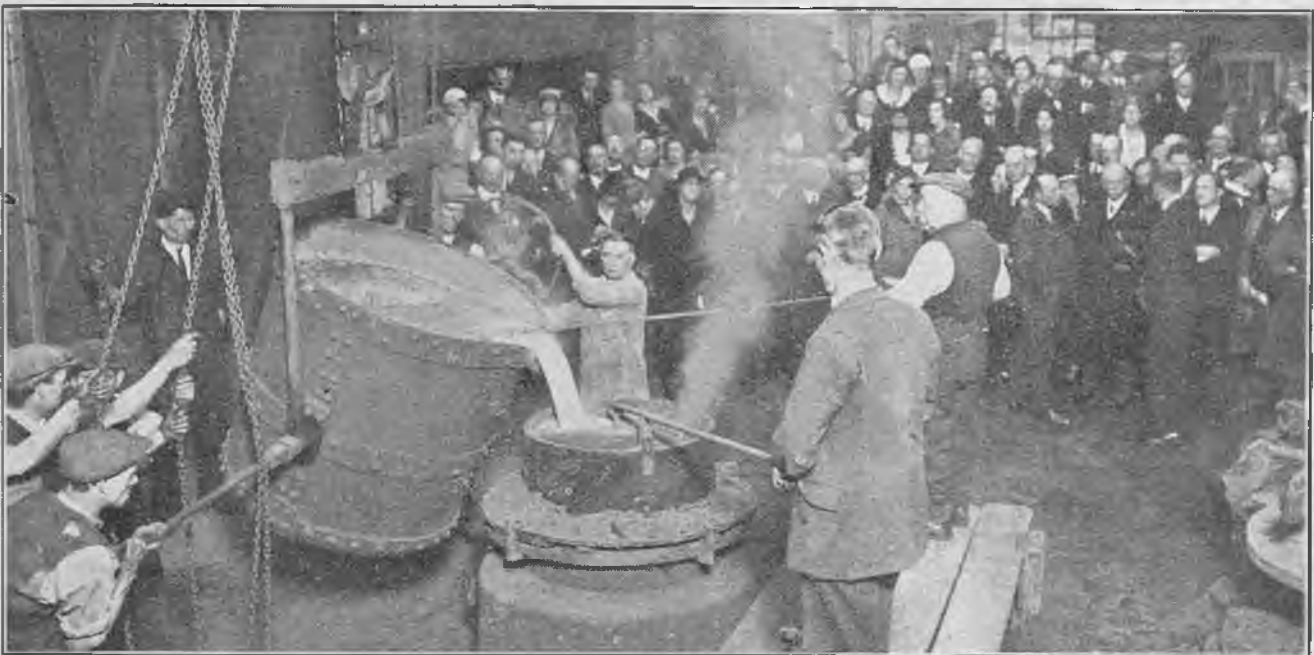
POURING THE METAL INTO THE MOULD AT THE RECASTING OF BOW TENOR.
